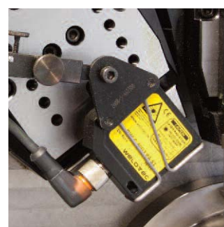
▲ Ejection control by means of laser
