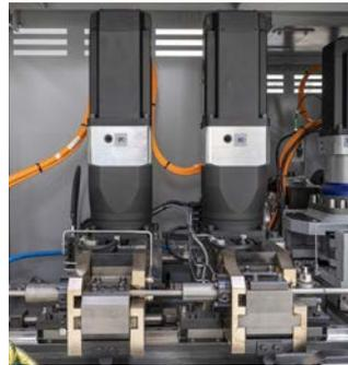
▼ The chain link blank transport passes the chain link to the bending station
