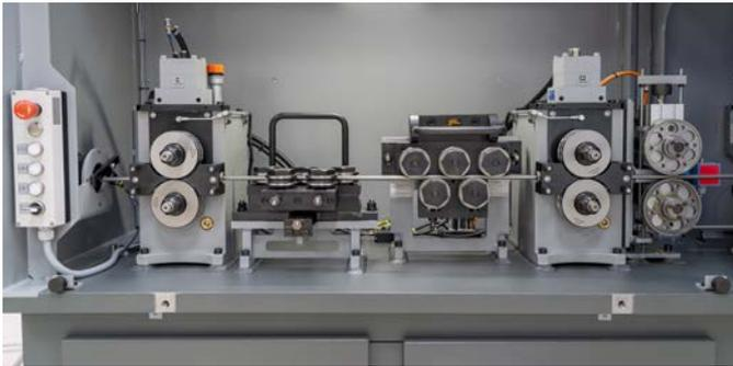
▼ Die forming device and notching device
