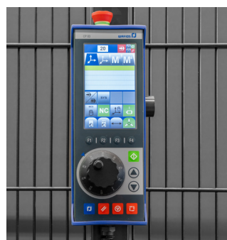
▲ Hand-held operating device with touchscreen
