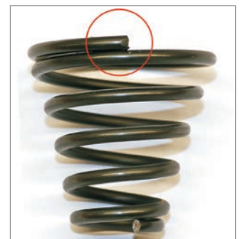
▲ Conical spring produced with motor-adjustable coiling pin holder (PTP coiling finger)
