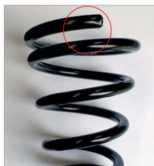
▲ Conical spring produced without PTP coiling finger
