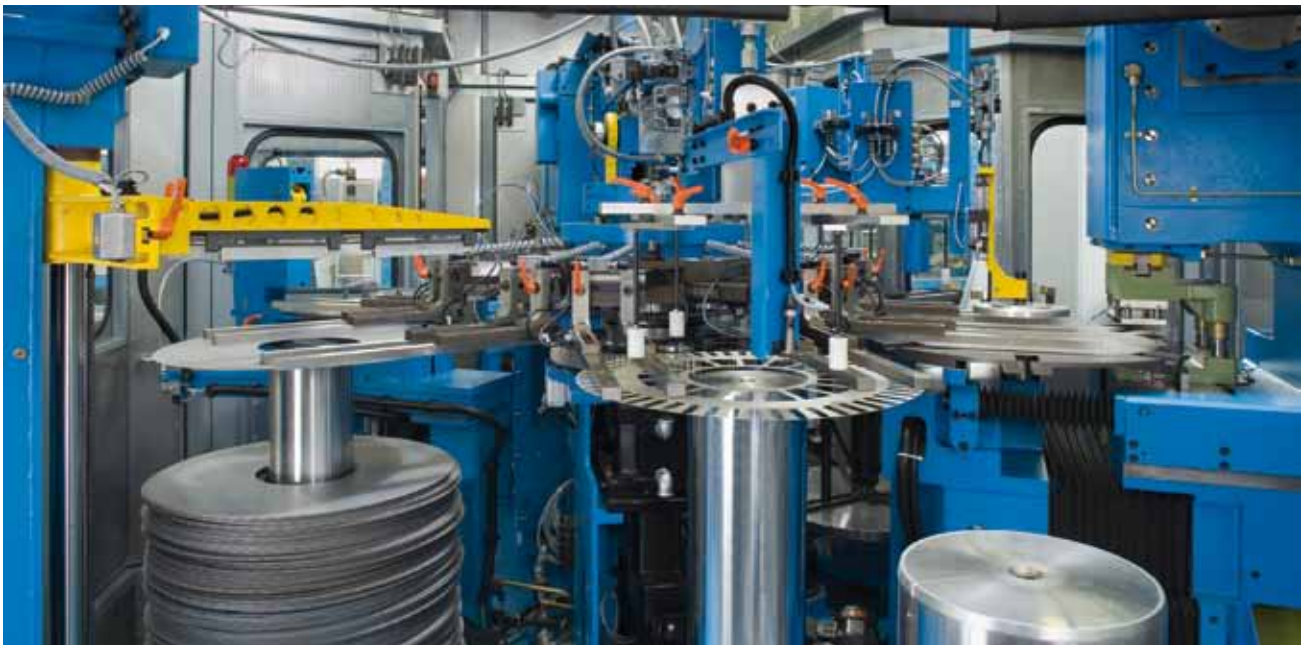
Fully automated notching line with circular transfer (spider) automation
