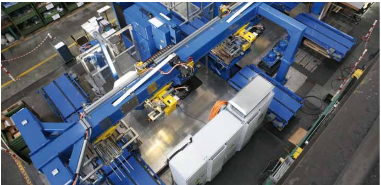
Fully automated notching line with linear automation
