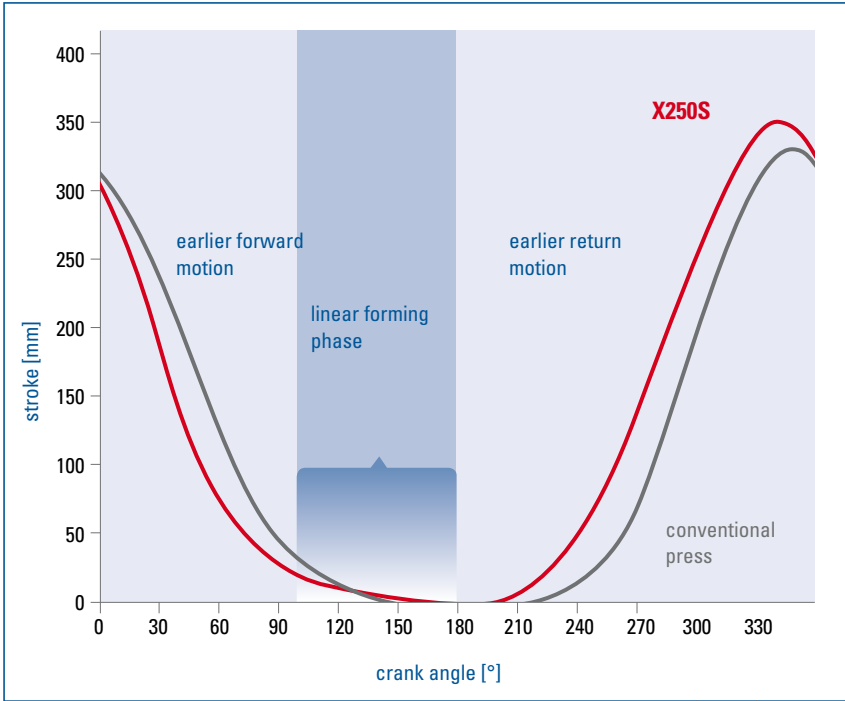
Slide motion of the X250S (red) as compared to a conventional impact extrusion press (gray).
