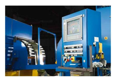
The electric motor lamination blanking line is operated using a Windows-based visualization system. It is easy, clear, convenient to use and user-friendly. Furthermore, parameters such as stroke, stroke rate, press force and shovel stroke etc. can easily be entered by the machine operator. The visualization and control system for the entire line has been developed by the Schuler Group.
