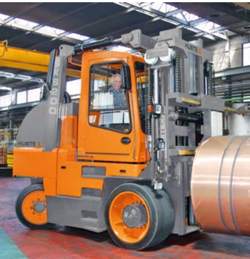
Gas-Kompaktstapler, Tragfähigkeit 20 t LPG-powered compact frontlift, capacity 20 t
