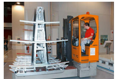
Multidirectional Sideloaders handles PV-modules on an A-stillage
