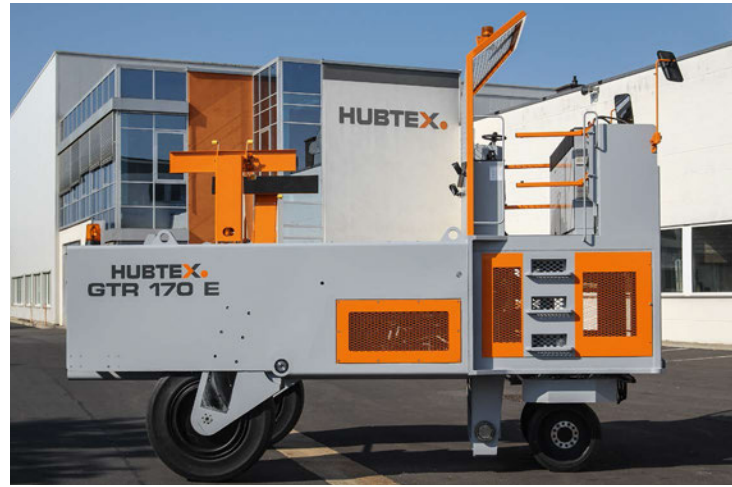
GTR for handling of LES stillages in a coating line
