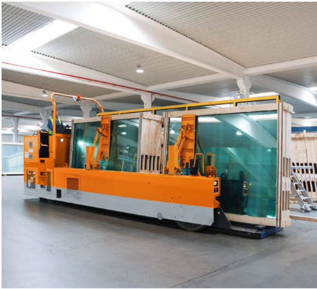
GTR 330 E transporting L-stillage with glass packs in end caps
