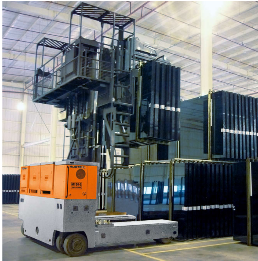
M 150 S0 stores glass packs in collars on two levels
