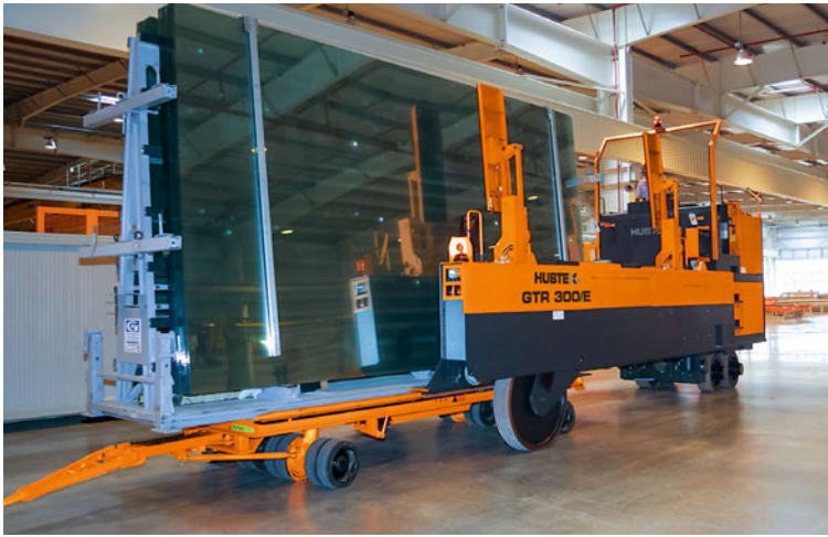
GTR unloading stillage from trolley
