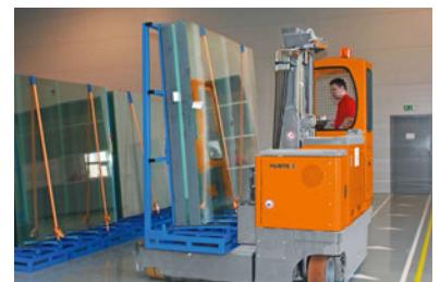
MQ 45 handles L-stillages with raw glass
