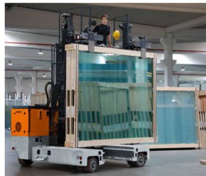
M 90 handling glass packs in end caps
