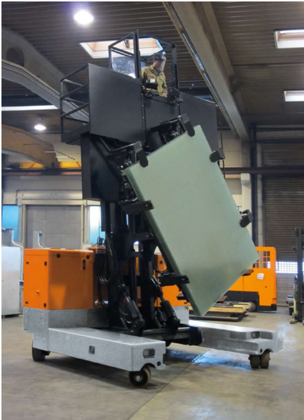
M 40 R (1-man version) for rotation of glass packs to feed a coating line
