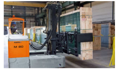
MQ 80 for handling glass packs in wooden crates up to 8 tons
