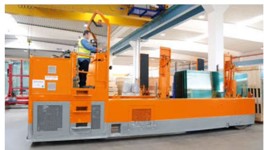
GTR 330 E feeding packing tables with unpacked glass packs
