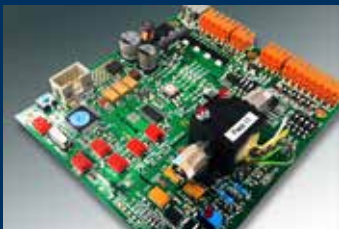
Electronic board with gas sensor
