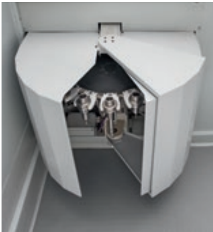
The machine can also be equipped with a rotating magazine (holding up to 16 tools) on the right-hand side to facilitate tooling operations.
